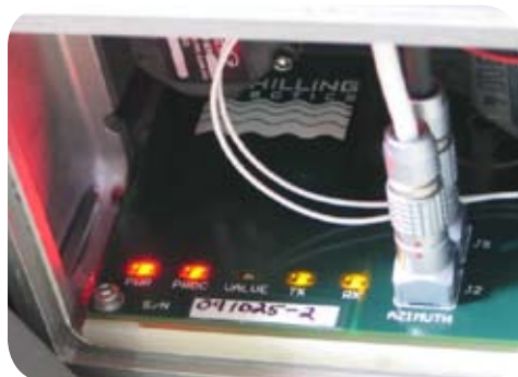
The in-arm slave electronics module features diagnostic lights that indicate processor health.
