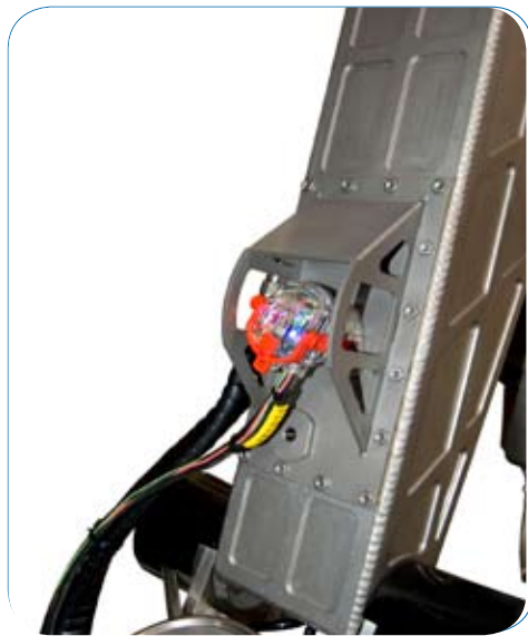
Diagnostic lights in the connector head indicate the status of electrical power delivery to the slave arm, master controller transmission to the slave arm, and slave arm responsiveness.
