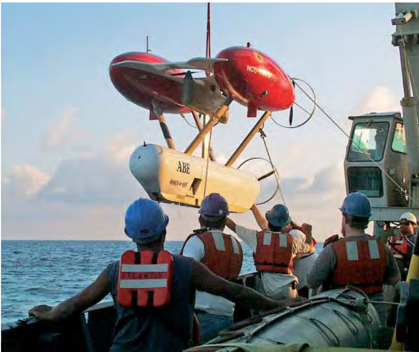
'Abe': Wood's Hole Oceanographic Institution's versatile deep sea vehicle. Picture courtesy of WHOI
